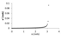
Figure 2- The relation between the emission angle of radiation  $\alpha$  from an isotropic point source in frame *S* and the angle  $\alpha'$  as seen by an observer in frame *S'*.
